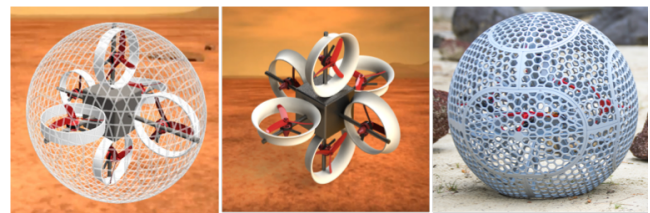
Figure 1: Left: Rollocopter concept art, including propellers, electronics (gray box) and the impact-resilient cage. Middle: hexacopter configuration of the propellers. Right: A Rollocopter prototype. The spherical cage allows to roll on flat terrains and to be impact-resistant, while the configuration of the propellers guarantees actuation in any direction.
